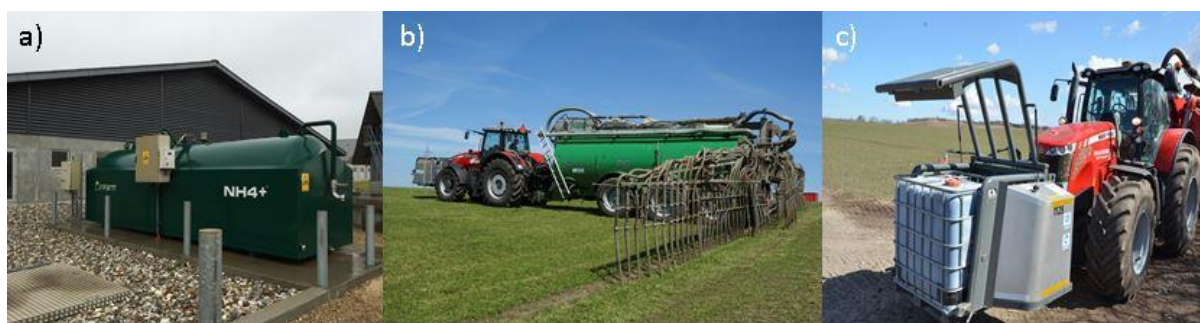
Figure 6. Acidification of slurry using sulphuric acid a) in house, Denmark (photo: Patrick Forrester) and b&c) during land application, Denmark (photo: Torkild Birkmose) using the SyreN system .
