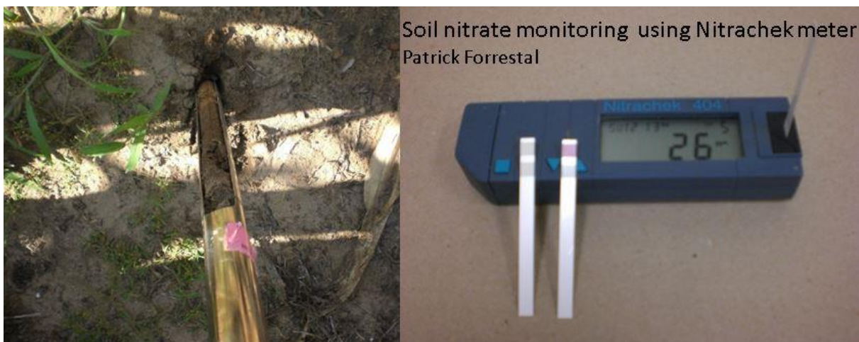
Figure 9. Soil nitrate measurement using nitrachek™ meter. Photo: Patrick Forrestal.
