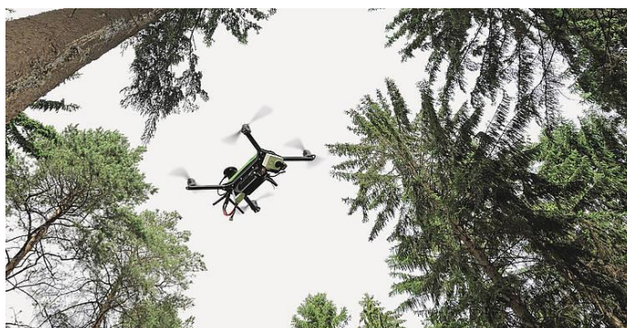
Fig. 2 Multicopter detecting barkbeetle infestation in Thuringia, Germany. Photo: © Carmen Rudolph
