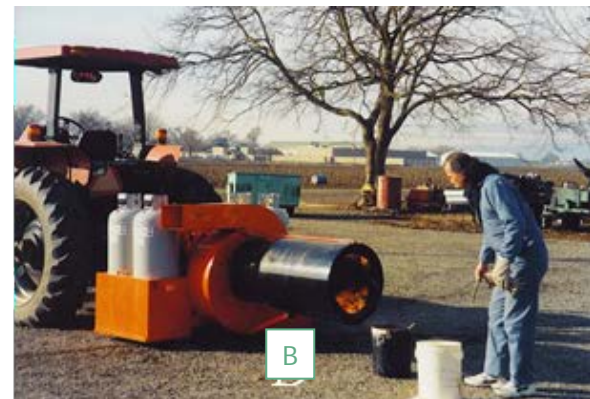
Fig. 3. (A) Upward-blowing wind machines (SIS system). (B) Horizontal hot-air blowers towed by a tractor (photo: R.L. Snyder)
