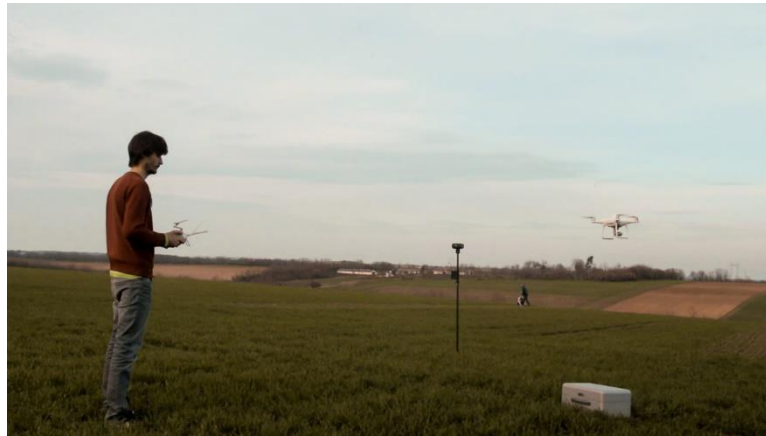
Figure 3. High precision RTK based crop monitoring enables farmers to realize site-specific input material applications (source: Discovery Center Kft)
