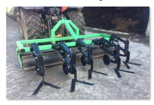
then weeds might not germinate and the crop can be sown through the dying mulch. At that stage I was afraid of another failure so I was not prepared to invest too much time and money into it, so I made a machine that might give an indication if it would work. It gave positive results! So I am now making a more permanent version of the machine - mounting the A shares on parallelograms with depth control wheels.
