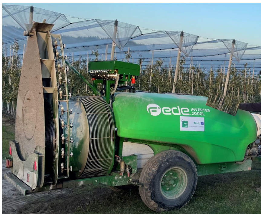
Figure 10: Fede precision agriculture sprayer with AI's crop sensing technology during field trials at 40 ha apple farm PAWLAK in Poland.
